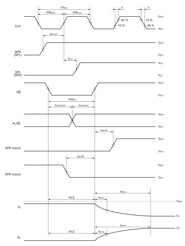
Vx refers to the final output voltage, tPLH2 and tPHL2 refer to the time required to an output precision level of 10 % (0.1 Vx); and tPLH3 and tPHL3 refer to the time required to reach an output precision level of 6 bits.
