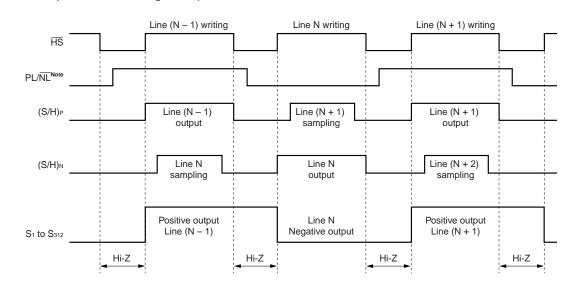
(3) Sampling and hold timing  $(R/\overline{L} = "L")$ S/ $\overline{D} = "L"$  (Dual Bank Arrangement)
